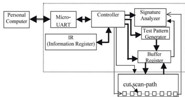
Fig. 1. Functional block diagram of the IC tester
