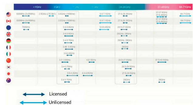
Figure 3. 5G low-frequency band distribution in various countries and regions of the world
