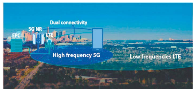
Figure 9. UE connectivity to LTE ng-eNB and 5G gNB in EN-DC mode [6]
