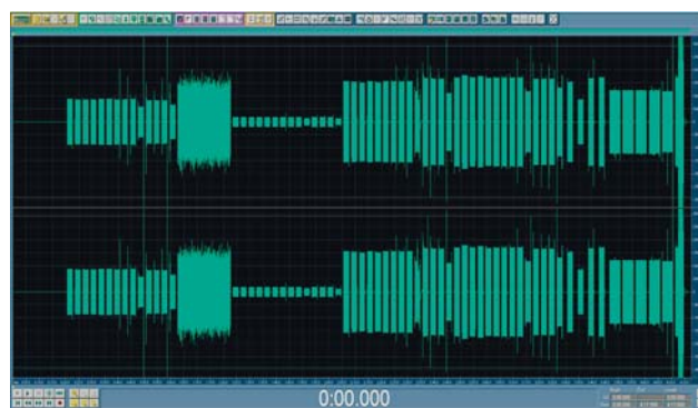
Fig. 3. Timing diagram of the output test signal for mode "A", 9 kHz, 64 QAM, immunity level "1"
