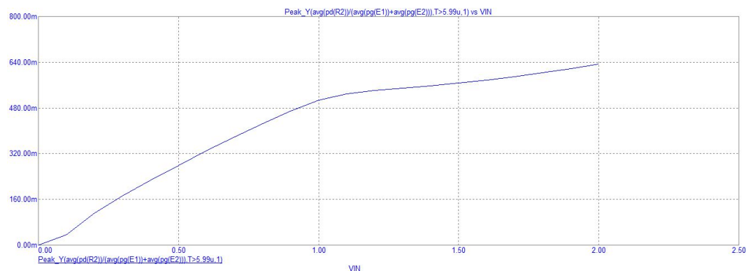
Fig. 1: The dependence of the efficiency on the signal amplitude in the amplifier W. Doherty
