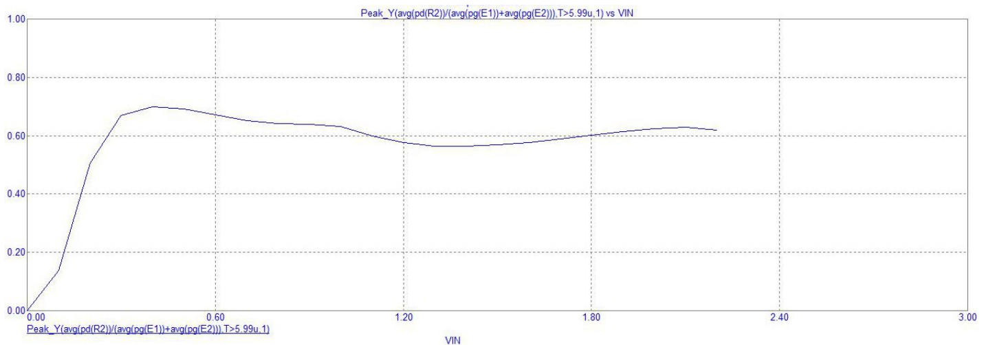
Fig. 3: The efficiency dependence on the signal amplitude in the W. Doherty amplifier with power supply mode automatic control in the main arm of circuit
