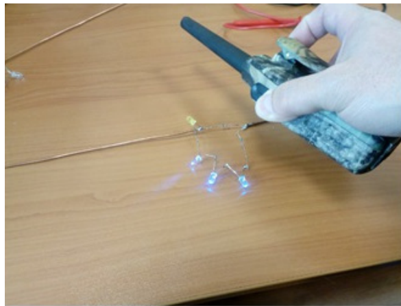
Figure 8. Remote power supply of LEDs at an angle between the plane of radiation polarization and the direction of the dipole antenna of 75 degrees. Radio frequency 150 MHz
