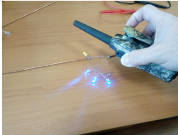
Figure 7. Remote power supply of LEDs at an angle of 60 degrees between the plane of radiation polarization and the direction of the dipole antenna. Radio frequency 150 MHz
