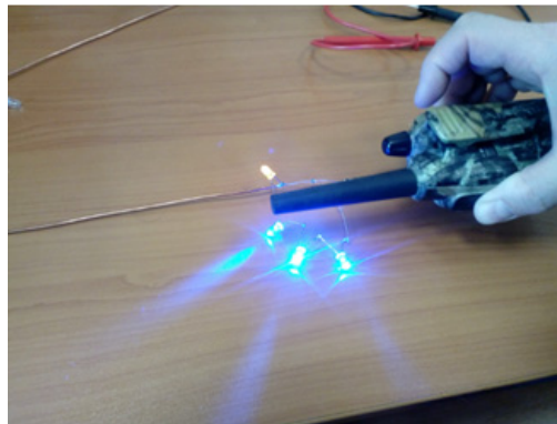
Figure 6. Remote power supply of LEDs at an angle between the plane of radiation polarization and the direction of the dipole antenna of 0 degrees. Radio frequency 150 MHz
